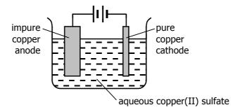
The loss in mass of the positive electrode was 50~g and the gain in mass of the negative electrode was 45~g.
