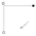
The ball is lifted to the same level as point *O*, with the string being just taut. It is then released from rest.
