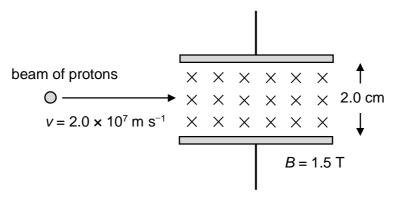
If protons travelling at  $2.0 \times 10^7$  m s<sup>-1</sup> pass through undeflected, what would be the direction and magnitude of the electric field?
