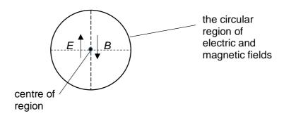
The deflections of the beam from the centre of the region produced by the electric field *E* and the magnetic field *B* acting separately are equal in magnitude.
