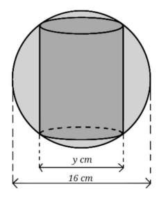
A cylinder of diameter *y cm* is inscribed in and is to be cut out of a plastic sphere of diameter 16 *cm*.
