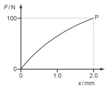
What could be the value of the elastic potential energy stored in the wire when it is stretched to point P?
