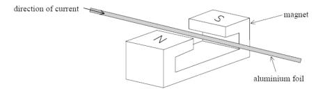
When a current is passed through the aluminum foil in the direction shown, the foil is deflected.
