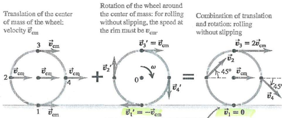
Figure 10: Pure Rolling Motion
