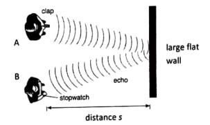
Observers A and B stand at equal distances from a large flat wall. Measure and record the distance s between the observers and the wall with a measuring tape. Observer A first claps the two blocks of wood to produce a loud sound. He continues to clap every time an echo is heard (the new clap must coincide with the echo of the previous clap). He makes 51 claps altogether.
