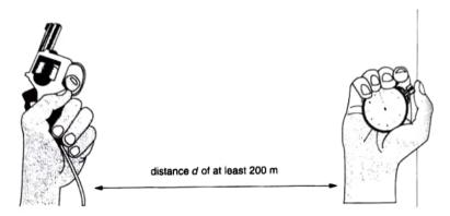
Observers A and B are positioned in an open field at a distance d (more than 200 m) apart. When A fires a starting pistol, B starts the stopwatch upon seeing the flash of the pistol and stops the stopwatch on hearing the gun shot. The time interval t is recorded. This is the time taken for the sound to travel the distance d.
