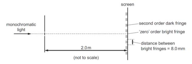
What is the path difference between the light waves from the two slits that meet at the second order dark fringe?
