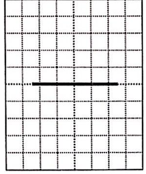
When the time-base is switched on, an internally generated saw-tooth voltage shown on the right is applied to the x-plates of the CRO.
