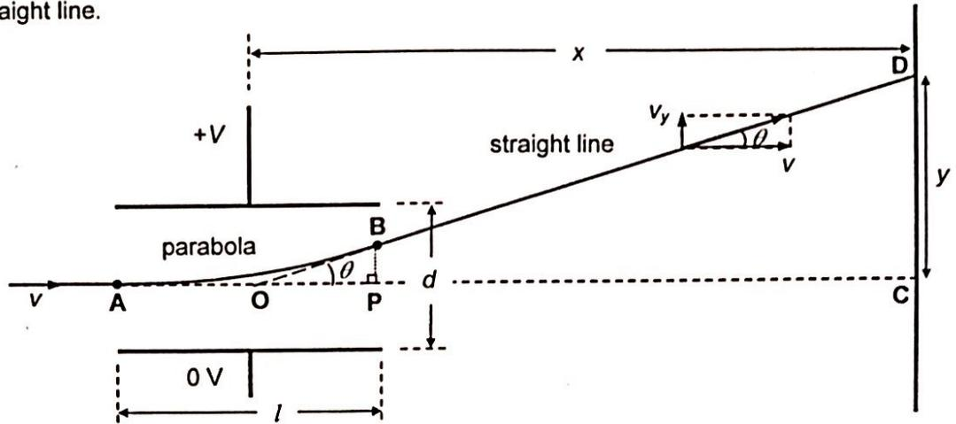
**Deflection of an electron beam through parallel plates**
