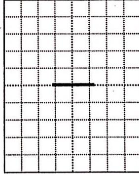
The screen on the right is obtained when the  $y$ -sensitivity is adjusted.  $y$ -sensitivity =  $1.0 \text{ V div}^{-1}$
