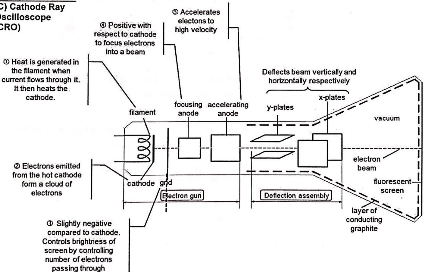
The main features of a cathode ray oscilloscope
