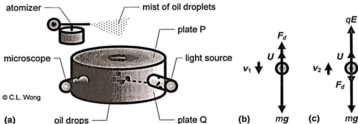
Fig. (a) shows a **simplified scheme** of the Millikan's oil-drop experiment, first used by Robert Millikan and Harvey Fletcher to determine the electric charge of the electron in 1909. By measuring the terminal speeds of the oil droplet between the plates, its electric charge can be measured. Robert Millikan was awarded the Nobel Prize in physics in 1923.
