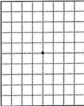
When a d.c. voltage is connected to the y-input, the spot of light is deflected as shown. The CRO commonly found in the laboratory are already calibrated.  $y$ -sensitivity =  $2.0 \text{ V div}^{-1}$
