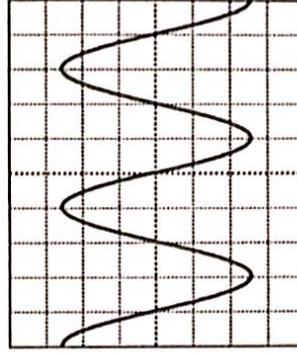
The same a.c. voltage is applied to the y-input but the time base is adjusted.  $\text{time-base} = 2 \text{ ms div}^{-1}$
