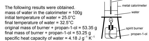
Use these results to calculate the experimental enthalpy change of combustion for propan-1-ol.
