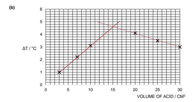
Draw 2 best-fit straight lines and extrapolate both lines to find volume of acid required to completely react with NaOH.
