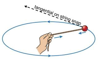
Tension in the string provides the centripetal force to keep the ball in circulation motion.
