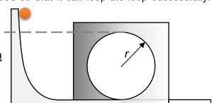
Resultant force of normal contact force by track on marble and weight provides centripetal force:
