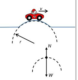
**Note:** it is "easier" for a car to lose contact for a small radius, making for an uncomfortable "bump". This is why larger, flatter speed bumps are more forgiving than very small and rounded ones.
