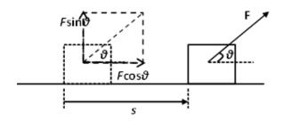
Only the component of the force along the displacement does work.
