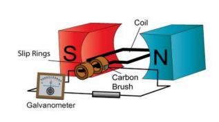
When coil is rotated at a uniform angular velocity,  $\omega$ , then,
