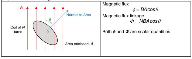
**Faraday's law** – the magnitude of the electromotive force induced ion a conductor is proportional to the rate of change of magnetic flux linkage of the conductor.
