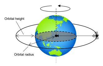
Geostationary satellites allow transmission of signals between two regions at all times because the satellite will remain within "line-of-sight" of ground-based transmission and reception equipment.
