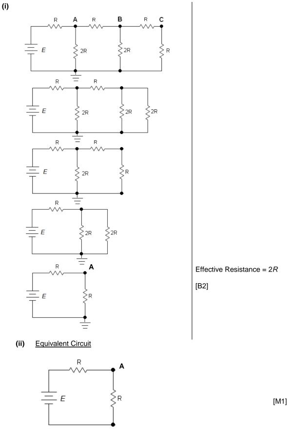
Emf E is divided equally between the two resistors R.
