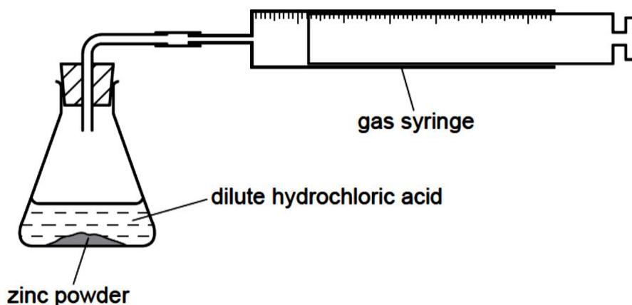
The volume of gas produced was measured every minute for six minutes. The results are shown in the table below.
