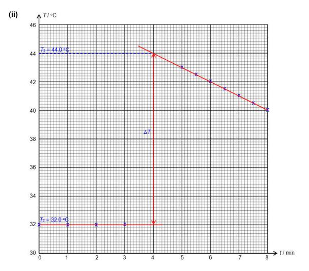
(iii) Minimum temperature,  $T_2$ , at t = 4.0 min is 32.0 °C.
