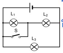
When swortch S is cloned, Lamp Li is typossed. Since effective vestitance across Li and L2 has decreased, current fishing intress of L2 will browned and this intress of L2 also browned. Since current flowing tworch L3 remains constant, trightness of L3 venaling unchanged
