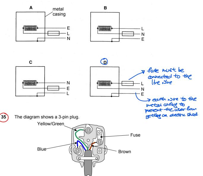
If the brown wire carries a current of 4 A when the appliance is switched on, what would be the currents in the yellow/green and blue wires?
