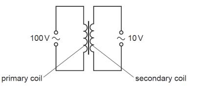
What are suitable numbers of turns for the primary coil and for the secondary coil?
