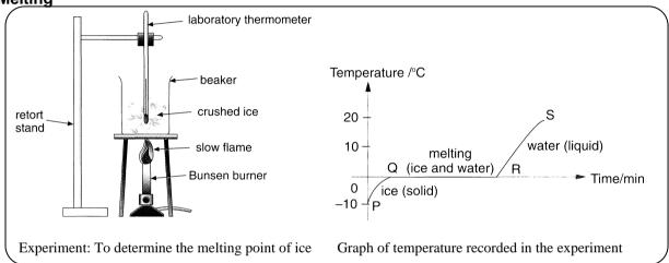
During the <u>change of state</u> from ice to water, there is <u>no change in temperature</u> even though heat is being absorbed.
