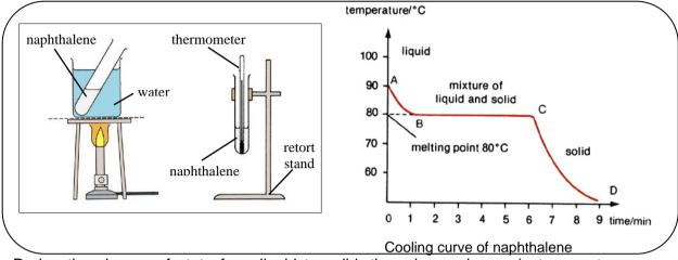
During the change of state from liquid to solid, there is no change in temperature even though heat is lost to the surroundings as the naphthalene cools. *Where does the energy come from?*
