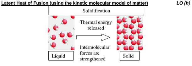
Heat is <u>released</u> as <u>intermolecular forces are strengthened</u> when the liquid atoms or molecules come together to form a solid. The atoms or molecules now take on a more ordered structure as compared to the less ordered structure of the moving liquid atoms or molecules. This explains why there is no change in temperature during solidification.
