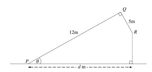
The diagram shows two rods PQ and QR, of lengths 12m and 5m respectively. The rods are fixed at Q such that angle  $PQR = 90^{\circ}$  and hinged at P so as to rotate in a vertical plane. The rod PQ makes an angle  $\theta$  with horizontal ground.
