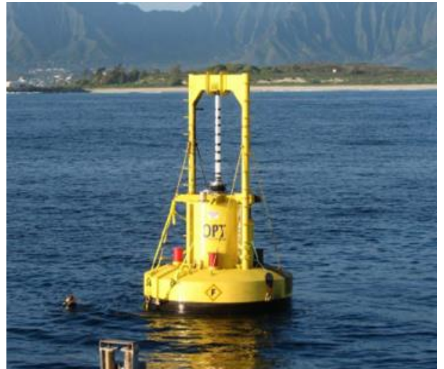
Rise and fall of a buoy generates 20 kW.
