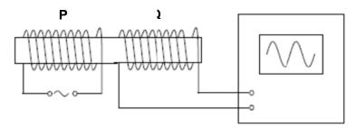
What would be the effect on the trace if the soft-iron core is removed?
