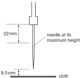
The oscillation is simple harmonic with a frequency of 4.5 Hz. The cloth that is being sewn is positioned 8.0 mm below the point of the needle when the needle is at its maximum height.
