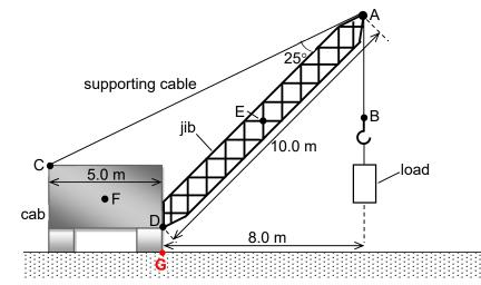
(ii) When the crane is just about to topple about G, the normal contact force on the left wheel just goes to zero.
