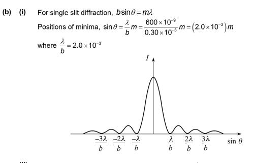
(ii) limiting angle of resolution for the single slit,  $\theta_{\min} \approx \frac{\lambda}{b} = 2.0 \times 10^{-3}$  rad
