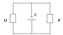
What is the change in power dissipated by P when the cell C is replaced with a cell with an e.m.f. of 24 V and an internal resistance of 1.0  $\Omega$ ?
