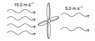
If efficiency of the turbine is 25%, what is the electrical power generated by the turbine?
