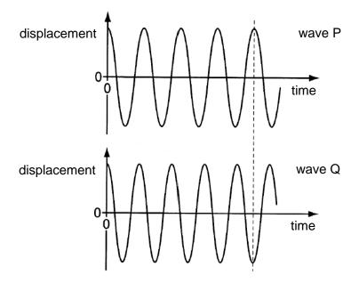
The frequency of Q is 125 Hz. The waves are in phase at time = 0.
