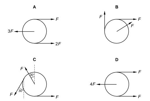
Check for  $\Sigma Fx \neq 0$  OR  $\Sigma Fy \neq 0$  for non-zero resultant force .
