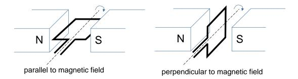
What is the maximum e.m.f. induced and the corresponding orientation of the coil?
