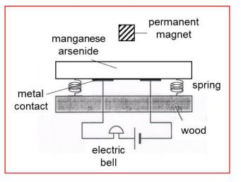
(b) When the surrounding temperature is 45 °C or higher, manganese arsenide becomes non-magnetic and is no longer attracted by the magnet.
