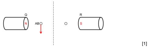
(c) [1] When current flows through the coil, <u>the magnetic field of the electromagnets interact with the magnetic field of the wire AB.</u>
