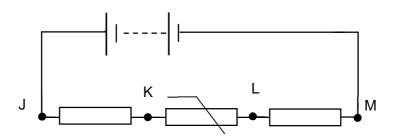
Which of the following best describes the potential differences between the points J & K and J & L when the temperature of the thermistor increases?
