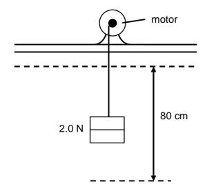
The efficiency of the motor is 20 %.
