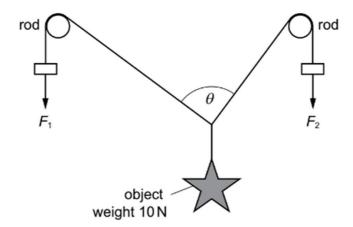
The object is held in equilibrium by the forces  $F_1$  and  $F_2$ . The object weights 10 N. There is negligible friction between the rods and cords.
