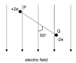
The electric field strength is  $1.5 \times 10^5 \text{ V m}^{-1}$ . The line joining P and Q is at an angle of  $55^{\circ}$  to the direction of the electric field.
