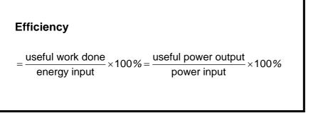
By the Principle of Conservation of Energy, the efficiency of devices cannot be more than 100%, and is almost always less than 100% in the real world as some energy will inevitably be dissipated in other forms alongside the desired output energy.
