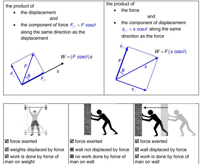
The S.I. unit for work done is *joule* (J). 1 J is defined as the work done when a force of 1 N moves its point of application through a distance of 1 m in the direction of the force.
