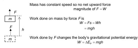
**Note**: The constant speed ensures that the kinetic energy remains constant; and that the work done by the force does not transfer energy to or from the body's kinetic energy. The work done in this case affects purely the gravitational potential energy only.
