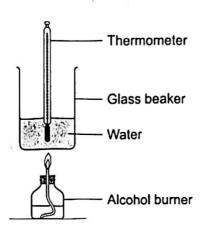
Some methanol was placed in the alcohol burner. The initial temperature of the water was measured.
