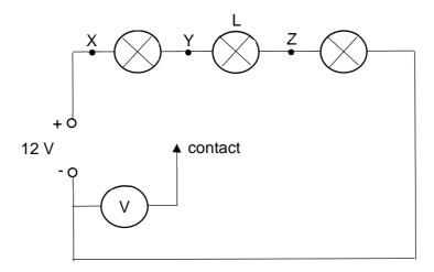
To test the circuit, the contact is connected in turn to points X, Y and Z. The lamps **do not light up** because lamp L has a broken filament.
