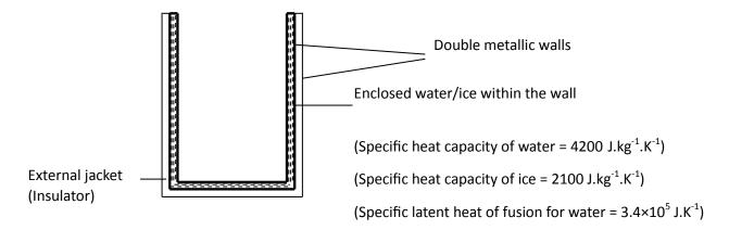
The mass of enclosed ice is 50 g and the initial temperature of the cup is -4°C. 330 g of drinking water at an initial temperature of 25°C is poured into the cup.
