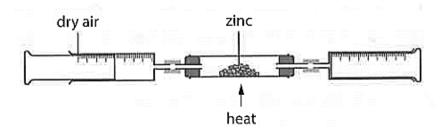
During the reaction, a sample of 250 cm<sup>3</sup> of air was used.
