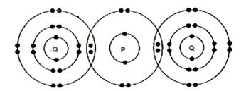
What are the electronic structures of atoms  ${\bf P}$  and  ${\bf Q}$  before combining together to form the above molecule?
