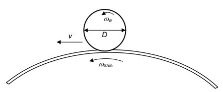
For a wheel of diameter *D* and angular velocity of  $\omega_{W}$  moving at speed *v* along a curved rail of radius *R*,
