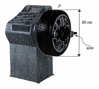
An important aspect to having a smooth car ride is to ensure the wheels are well balanced. To do that, the wheel is first mounted on the machine and rotated. The machine will then automatically calculate the weight and location of the balance counter weights to ensure that there are no heavy spots on the tyre.
