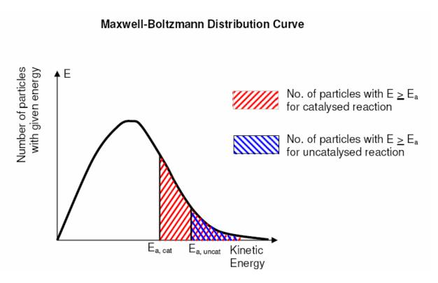
$E_a$  is lowered due to an alternative reaction pathway. Number of reactant particles with  $E \ge Ea$  increases. Hence, number of effective collisions per unit time increases. Hence, rate of reaction increases which causes an increase in iron overload in the liver, This aggravates the patient's condition.
