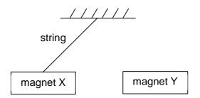
Magnet X has a weight of W. The magnetic force by magnet Y on magnet X is P. The tension in the string is T.
