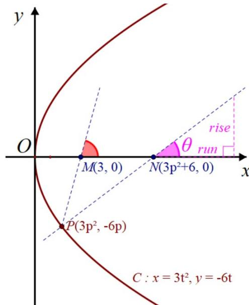
$\therefore$  Gradient of  $PN$  is given by  $\frac{\text{rise}}{\text{run}} = \tan \theta$ ,
