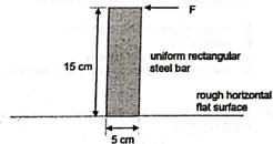
Which expression calculate the force F required to just tilt the steel bar from the horizontal surface?
