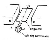
The split-ring commutator reverses the current in the coil as the coil rotates. If the coil is rotated 360° from the position shown, how many times is the current in the coil reversed?
