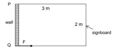
If the mass of the signboard is 60 kg, what is the normal reaction, F, exerted by the wall at Q?
