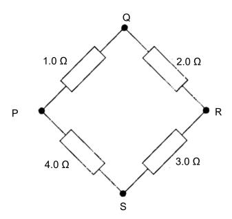
Between which two points would the resistance of the circuit be the greatest?
