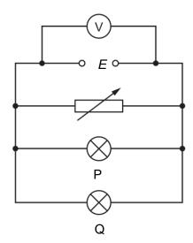
The resistance of the variable resistor is reduced. What happens to the brightness of the lamp?
