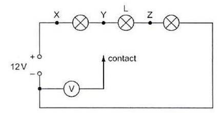
To test the circuit, the contact is connected in turn to points X, Y and Z. The lamps **do not light** because lamp L has a broken filament.
