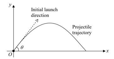
A projectile is launched from the origin with an initial velocity of u ms<sup>-1</sup> at an angle  $\theta$  radian above the horizontal, where  $0 < \theta < \frac{\pi}{2}$ , as shown in the diagram above.
