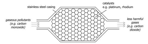
A **catalytic converter** is a device fitted in motor exhausts to facilitate the removal of air pollutants by \_\_\_\_\_allowing various air pollutants to react with each other \_\_\_\_\_ through a series of \_\_\_\_redox \_\_\_\_ reactions, forming less harmful products.
