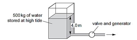
At high tide 500 kg of water is stored to a height of 4.0 m. When the valve is opened the container empties in 5.0 s and the generator operates with an efficiency of 40%.
