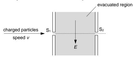
Uniform magnetic and electric fields are applied in the same evacuated region, with the electric field E in the direction shown. The particles continue to exit through slit  $S_2$ .
