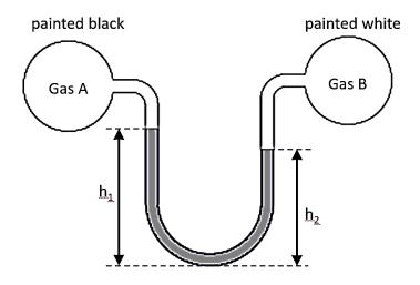
(a) Given that  $h_1 = 28.0$  cm and  $h_2 = 20.0$  cm and Gas A is at 772 mmHg, calculate the pressure of Gas B in mmHg.
