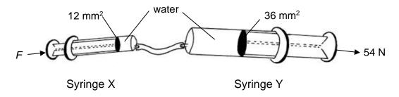
What is the input force F required to produce an output force of 54 N on syringe Y?
