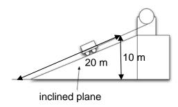
The motor has an average power of 100 W. What is its efficiency?
