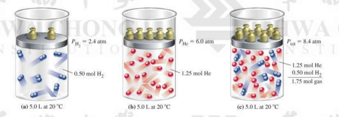
Figure 3 – Illustration of Dalton's Law of Partial Pressures
