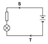
What are the directions of conventional current and electron flow in this circuit?
