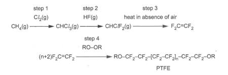
Step 4 occurs via four separate reactions, A to D.
