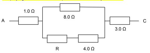
Since resistance between A and C is 8.0  $\Omega$ , resistance across parallel combination is 8.0 – 1.0 – 3.0 = 4.0  $\Omega$ . Thus, using the equation for equivalent resistance for resistors in parallel, we get $\frac{1}{4} = \frac{1}{8} + \frac{1}{R+4} = > \frac{1}{R+4} = \frac{1}{8} = > R = 4\Omega$
